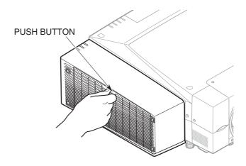
2 Open the filter cover and take out the used filter.
